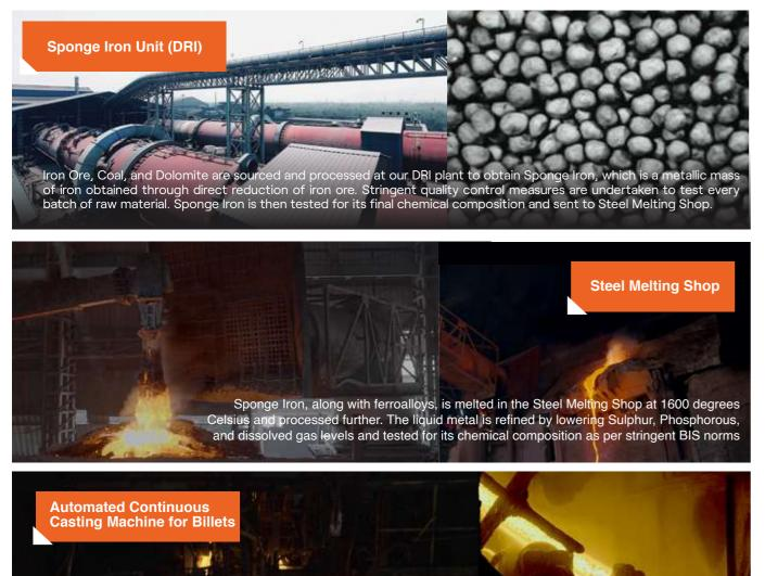
Molten Metal is passed through Automated Continuous Casting Machine for producing Billets. The molten metal is solidified during the continuous casting process to obtain high quality defect-free Billets to manufacture long steel products.
